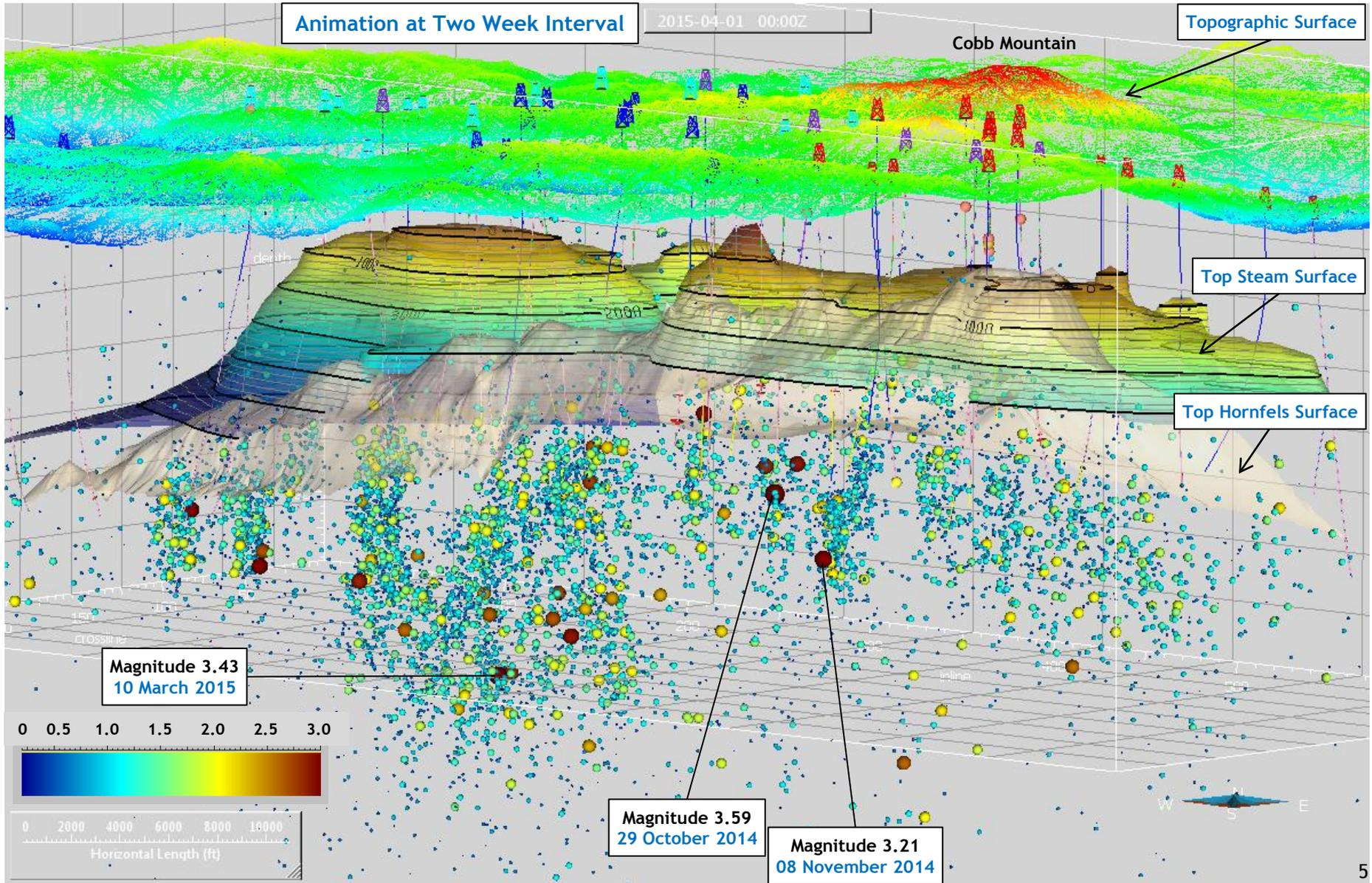
**The Geysers: Field-wide Steam Production, Water Injection and Seismicity
