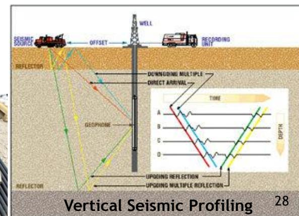
Vertical Seismic Profiling
