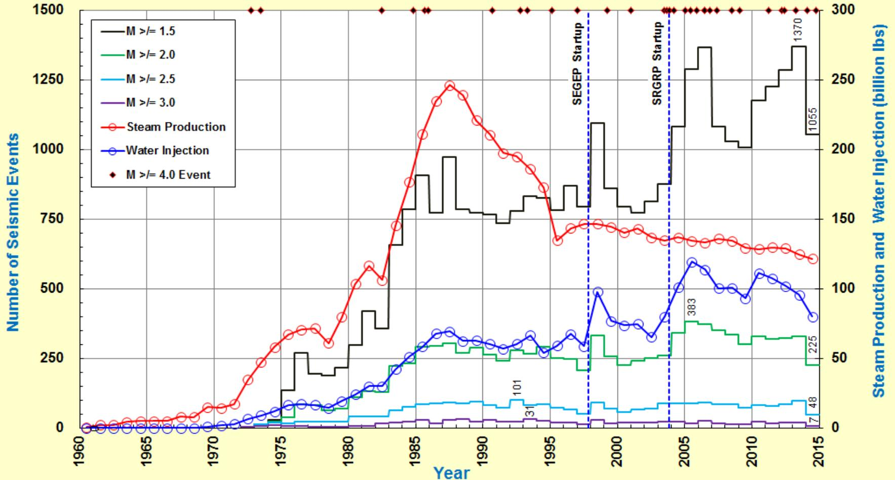
**The Geysers: Field-wide Water Injection and  $M \geq 1.5$  Seismicity
