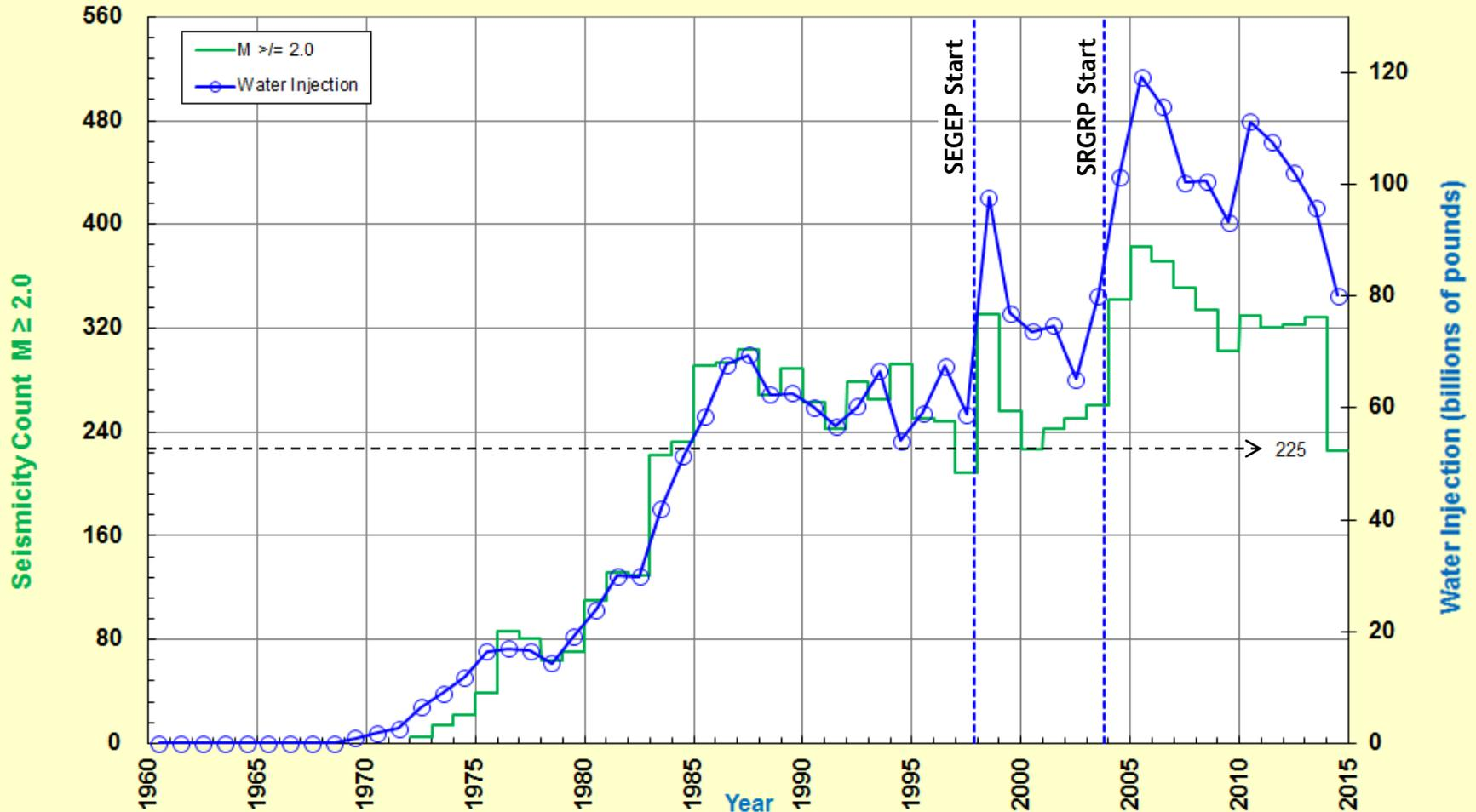
**The Geysers: Field-wide Water Injection and  $M \geq 2.5$  Seismicity
