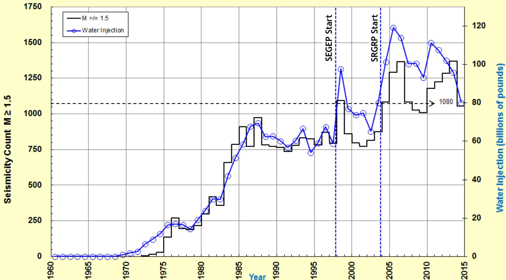
The Geysers: Field-wide Water Injection and  $M \geq 2.0$  Seismicity
