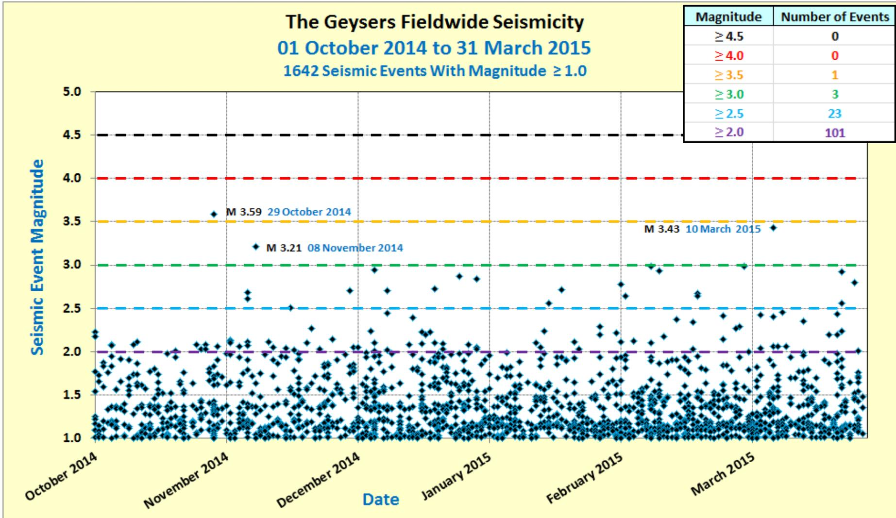
**Field-wide Seismicity Analysis**
