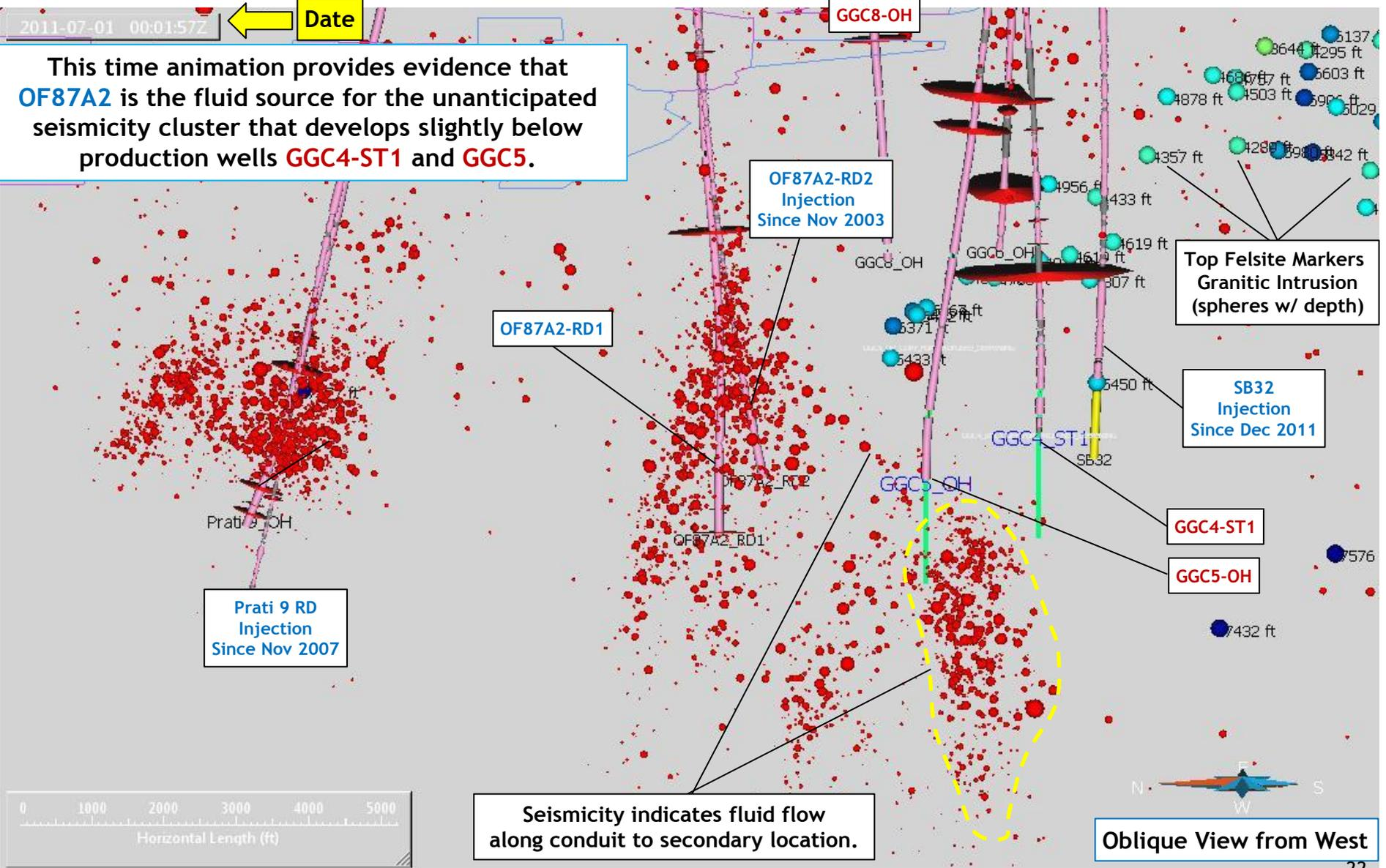
This time animation provides evidence that **OF87A2** is the fluid source for the unanticipated seismicity cluster that develops slightly below production wells **GGC4-ST1** and **GGC5**.
