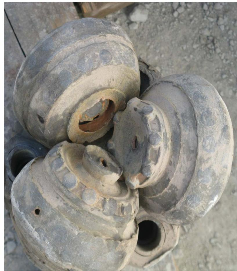
Prati 32 final bit condition after 105' of air drilling for 17 hours to TD (11,134').
