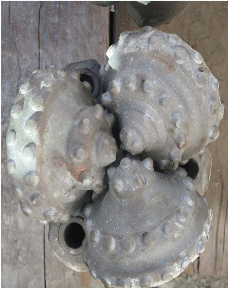
Average bit condition after 300' of air drilling for about 30 hours at the Geysers.
