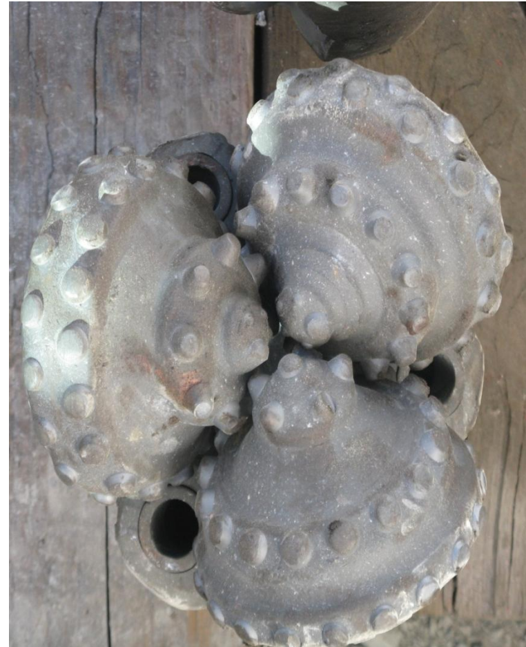
Average Bit Condition after 300' of drilling at the Geysers where temperatures are 450 °F
