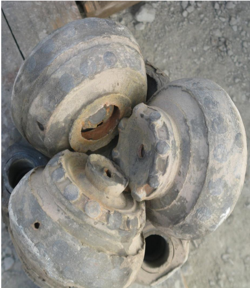
Final Bit from Prati 32 (11,134') after 100' of drilling where Temperatures are 750 °F
