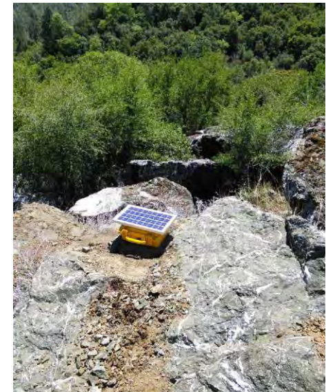
Sensor Installation on Rock Outcrop
